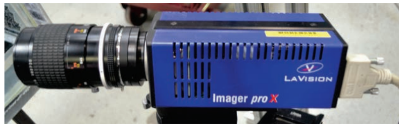
Figure 4.8: Imager ProX CCD cameras used for PIV measurements.
