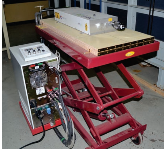
Figure 4.7: Nd:YAG laser used for PIV measurements.
